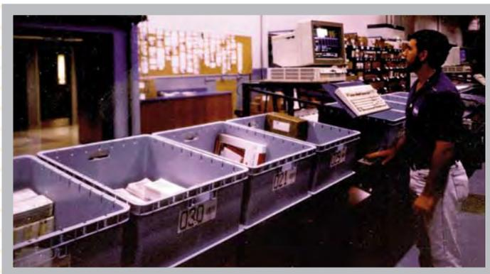
During both picking and replenishing, the operator is prompted by the PC, lighttrees, and sortbars for a virtually paperless system.
