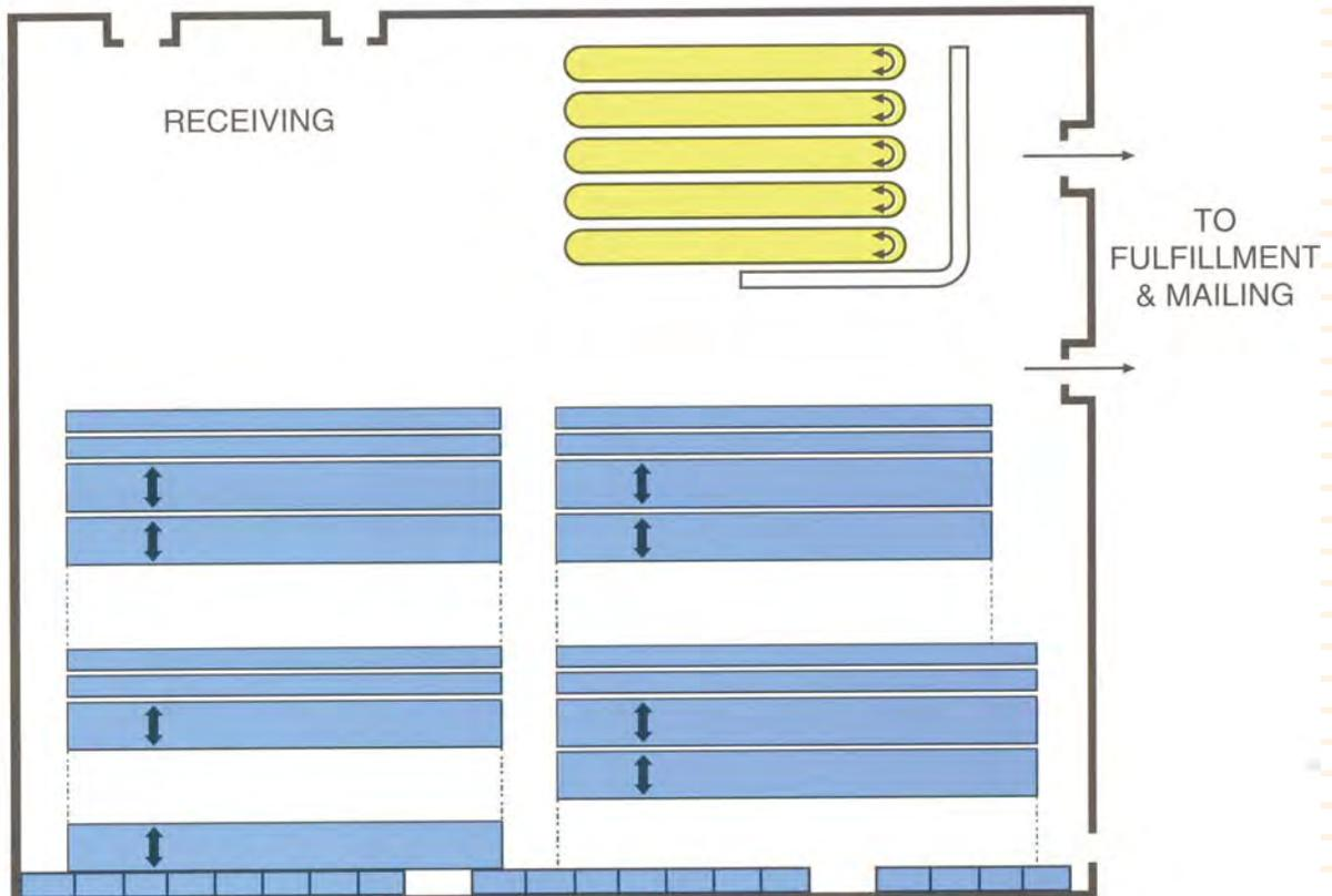
To open an aisle, an operator simply hits the “open” button on a carriage’s control panel. The carriages stop within a fraction of an inch.
