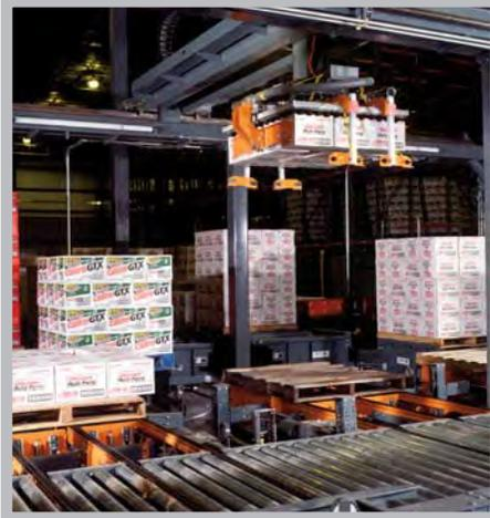
**Left:** White's pallet carousels with Alvey's gantry robot build mixed pallets for shipment to each store.
